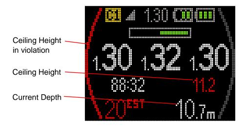
When the current depth has been shallower than the ceiling height for more than 2 minutes, the ceiling violation will be shown with a full red curve on the left as well as the normal 'Ceiling Violation' warning across the display.
