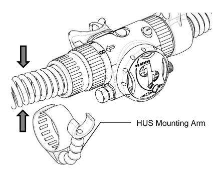
2. Whilst compressed, thread the HUS mounting arm over the hose
