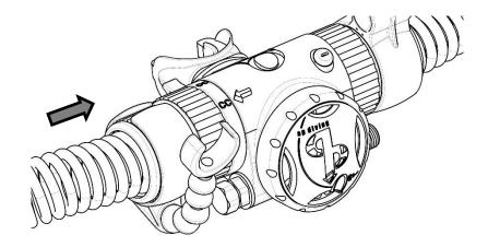
4. Prior to mounting the HUS, it is recommend that the HUS cable is wrapped around the convoluted hose to prevent the cable from becoming a snag hazard. Depending on the rebreather setup and hose lengths, it may be necessary to wrap the cable around several times to take up extra length.
