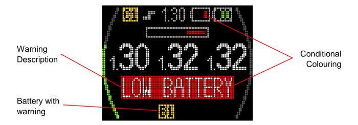
The HUS displays which Controllers (or Batteries) are generating the warning as well as conditionally colouring the related information red – in this case the PPO<sub>2</sub> values.
