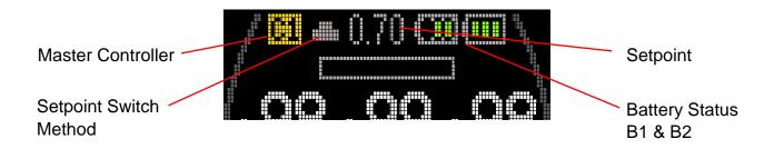
The Setpoint Switch Mode icons are shown below, manual, automatic, gradual and forced low (respectively). If the diver selects to switch to Open Circuit on the handset, the 'OC' symbol will replace the setpoint mode icon.
