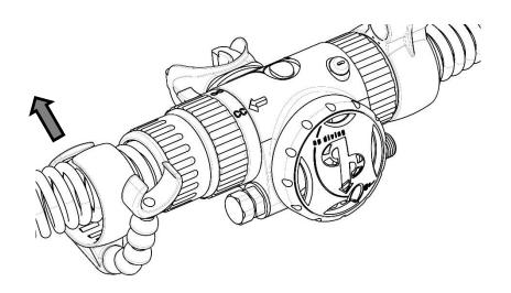
3. Slide the mounting arm onto the hose fitting where it should snap into place
