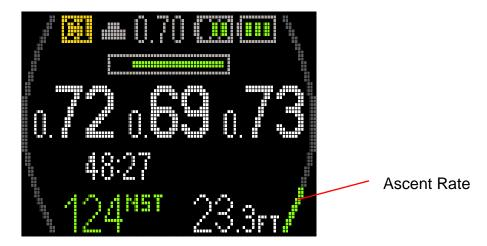
When ascending at a rate of less than 5m/min the bar graph will be green.
