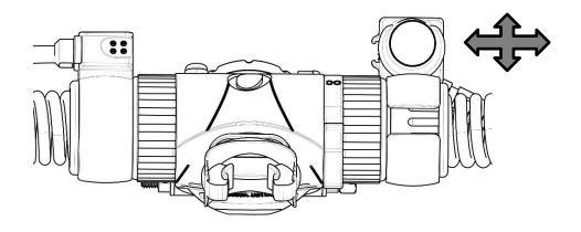
The nature of the articulated arm means that very fine position adjustments are possible, and alterations can be made at any time prior to or during the dive. The HUS arm length can be adjusted by removing or adding push-together sections.
