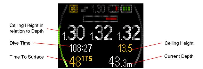
The time to surface and ceiling height are shown in yellow, highlighting the decompression obligation currently in place. The HUS also shows a graphical representation of the ceiling height in relation to the current depth. This is the curve on the left of the display and is explained later in this manual.
