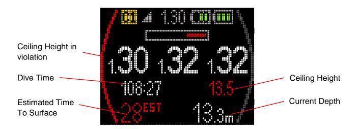
The estimated time to surface and ceiling height are shown in red, highlighting the fact that the decompression is now estimated due to the ceiling violation.
