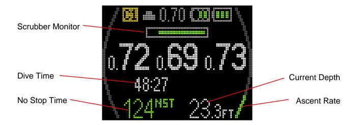
The no stop time is shown in green, meaning there is currently no decompression required. The scrubber monitor and battery status are also in green showing a good condition. All other information in this example are shown in white as they are all within the appropriate limits.
