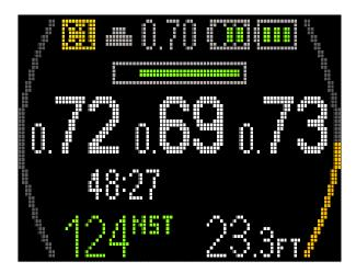
As the ascent rate increases the graphic extends higher and turns yellow when the ascent rate is between 5 and 10m/min.
