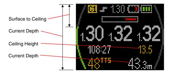
The green shows the 'Ceiling Height' in relation to the 'Current Depth'. This is continually updated throughout the dive once decompression is incurred and until no other stops are required, when the grey graphic will extend to the bottom of the screen.
